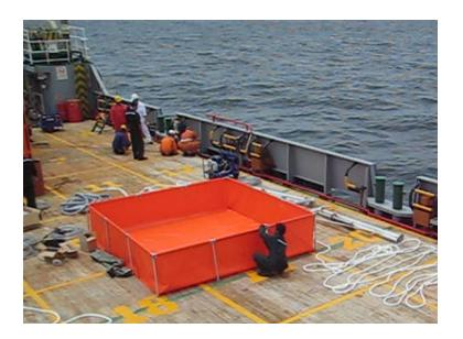
The STORAGE TANKs are self-supporting with a lightweight frame or the round one with pvc side supports and they are very easy to assemble
